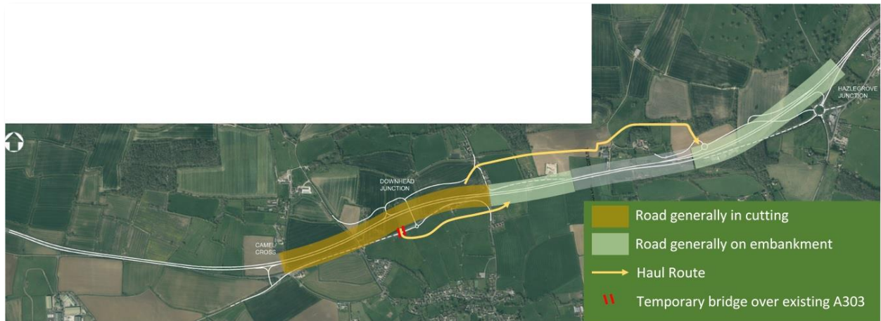
Figure 2.1 Earthworks haulage routes.
